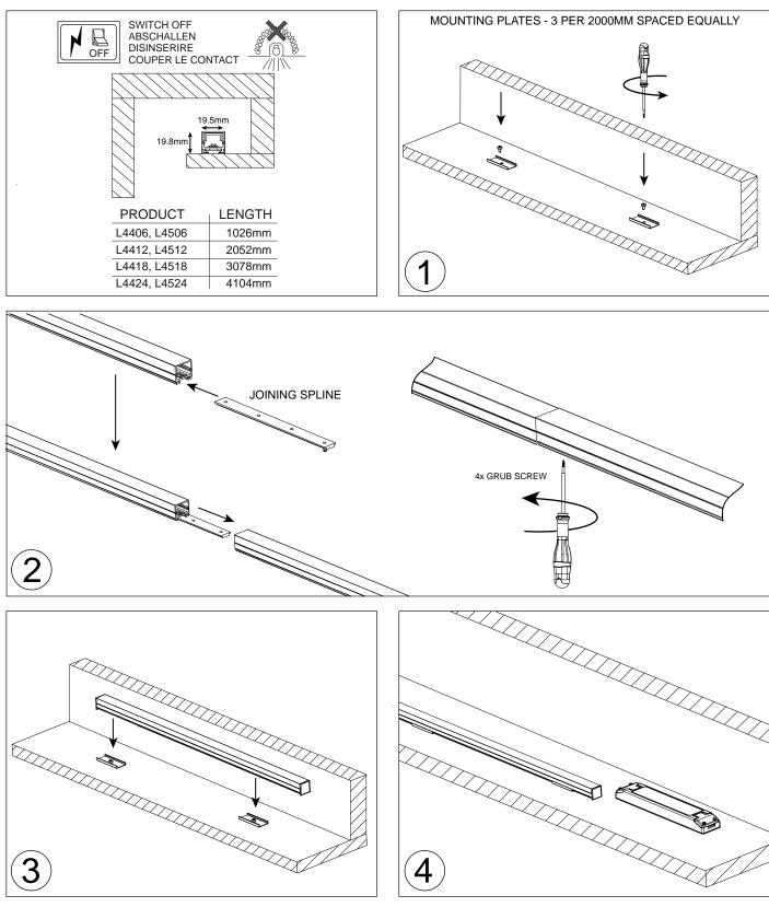
WARNING. SWITCH OFF MAINS BEFORE INSTALLING OR SERVICING
